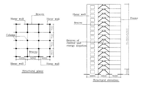
Fig. 5. Structural plane and elevation
