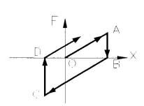
Fig. 3. Restoring force model of controlled brace
