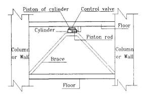
Fig. 1. Schematic of energy dissipation system
