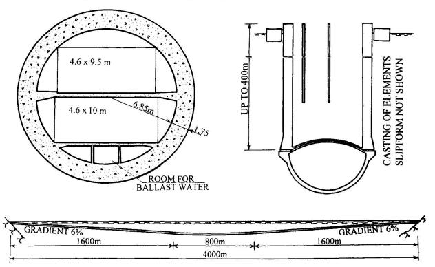
In the serviceability limit state the traffic load is very important. This load is at a maximum when traffic is brought to a standstill. It can be considerably reduced if traffic is not allowed into the tube whenever stoppages lead to undesirable deflections. The corresponding reduction in traffic capacity will be small. The ultimate limit state should be based on max. traffic load.
