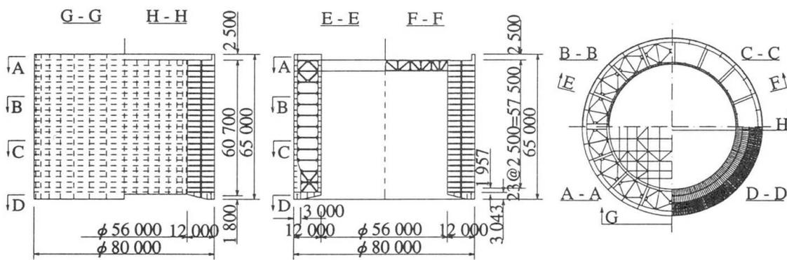
Fig.2 Structural Diagrams of 2P steel Caisson
