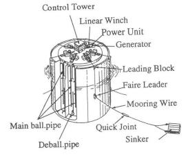
Fig.4 Concept of 2P caisson Equipment
