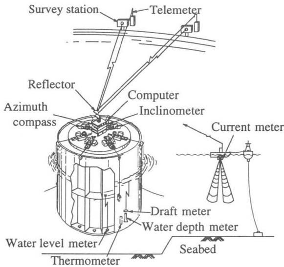
Fig.7 Layout of Monitor System
