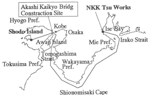
Fig.9 Towing route of 2P caisson
