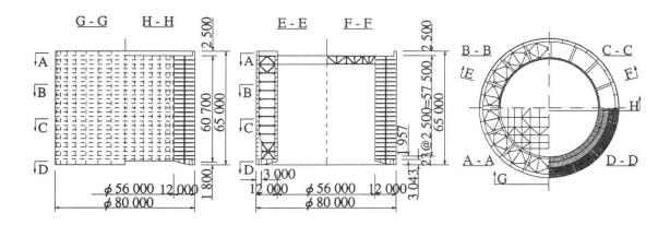
Fig.2 Strucutal Diagrams of 2P steel Caisson
