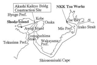
Fig.9 Towing route of 2P caisson
