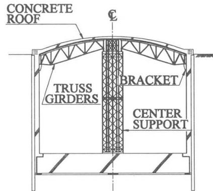
Fig. 9 Section of steel truss structure
