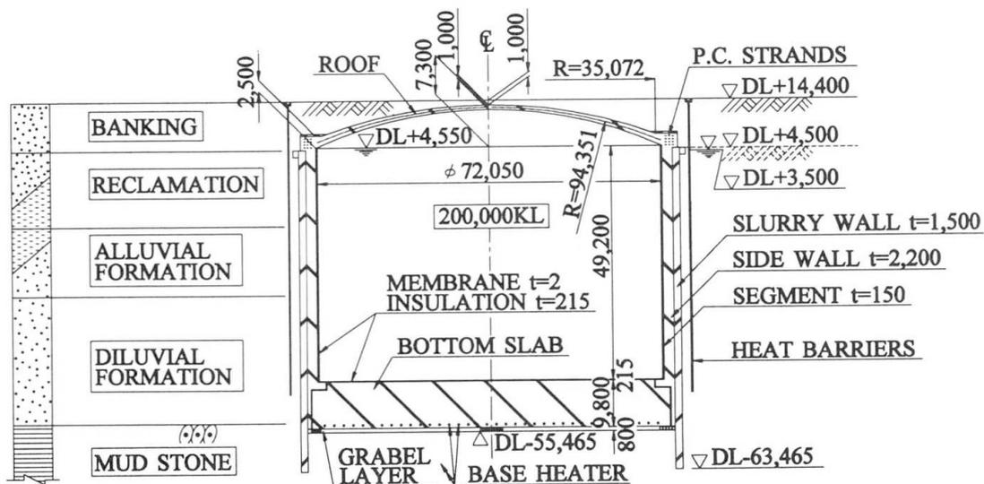
Fig. 2 Section of 200,000 kl LNG underground tank
