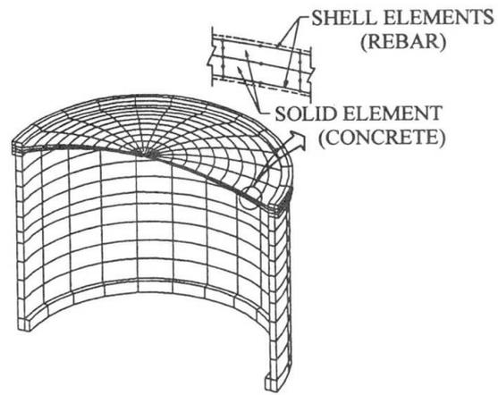
Fig. 4 Non-linear analysis model of underground tank
