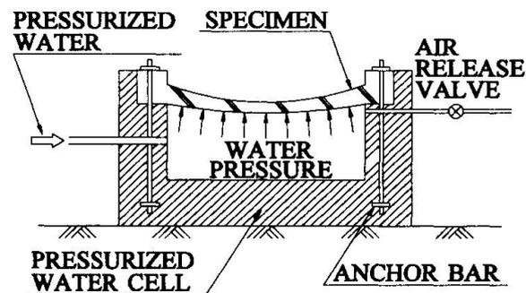
Fig. 3 Experimental model test of dome roof
