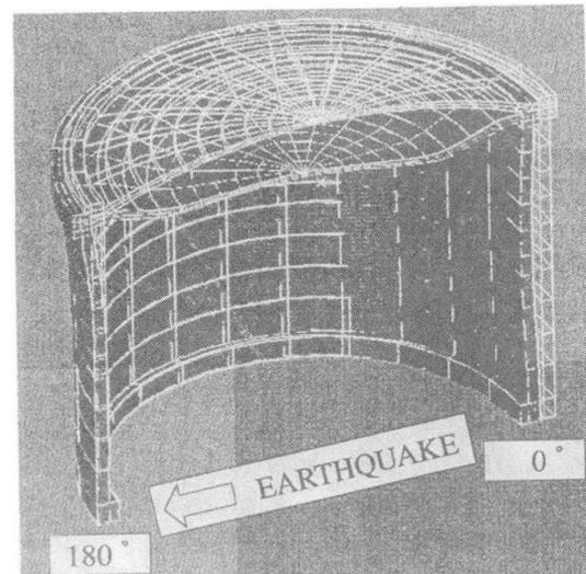
Fig. 5 Result of non-linear analysis (Deflection mode)
