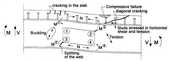
Fig. 4 Deformation at opening No. 3, engineering model
