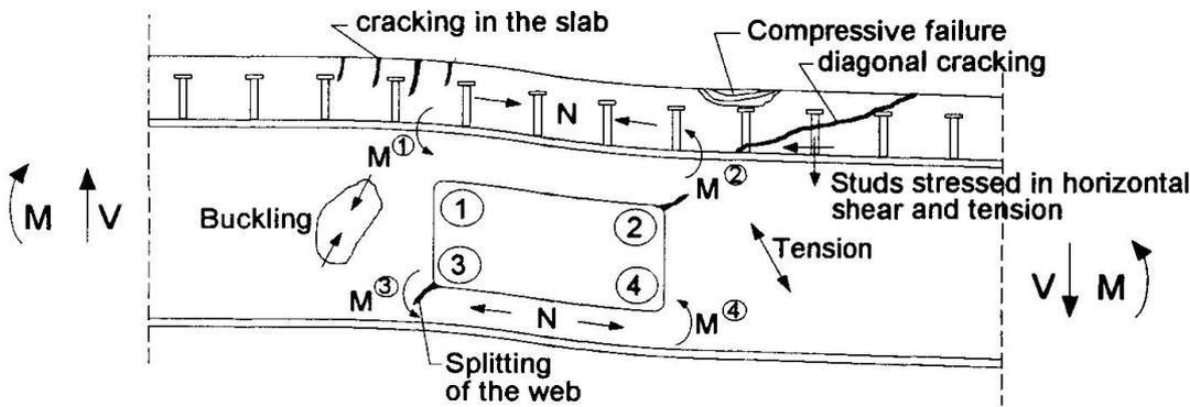
Fig. 4 Deformation at opening No. 3, engineering model
