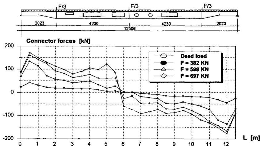
Fig. 3 Connector forces in the composite beam
