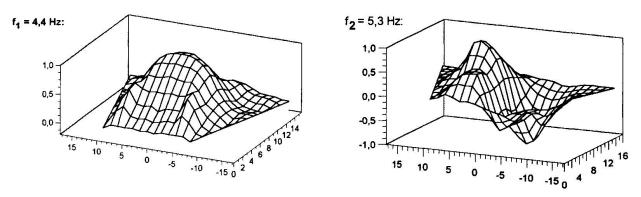
Fig. 5 First two shapes of the maximum acceleration of the slab
