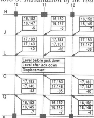
Figure 10 Results of measurement of bay 3
