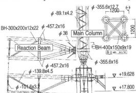
Figure 6: Joint detail of column and reaction beam
