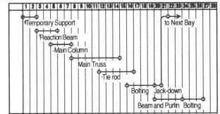
Figure 9: Construction schedule of main roof (for 1bay)
