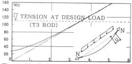
Figure 11: Relationship between elongation and tension
