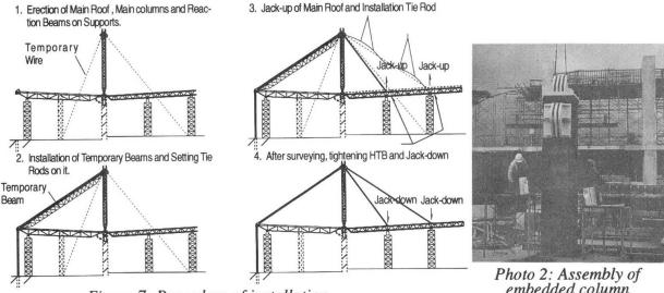
Figure 7: Procedure of installation
