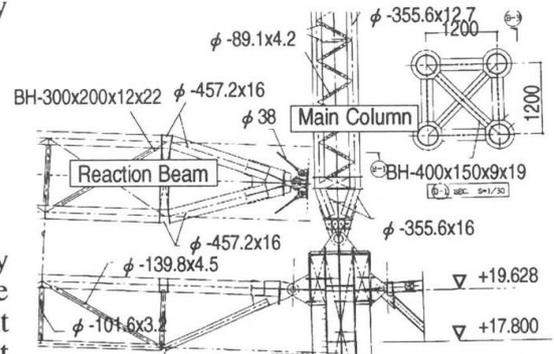
Figure 6: Joint detail of column and reaction beam
