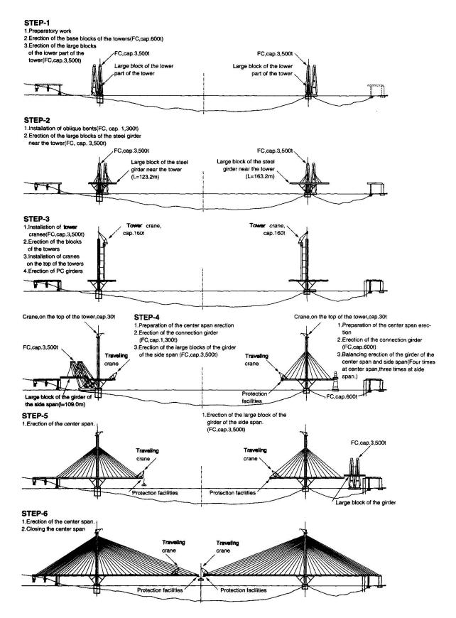
Fig. 4 Erection procedures of the Superstructure
