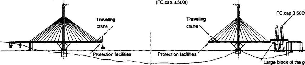
1. Erection of the large block of the girder of the side span. (FC, cap. 3,500t)
