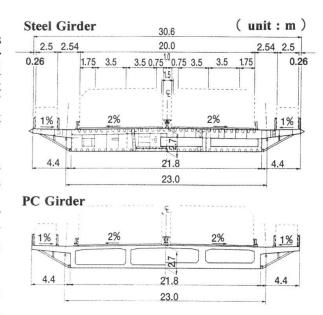
Fig. 3 Cross Section of Girder
