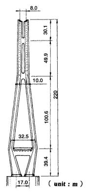
Fig. 2 Front View of Tower
