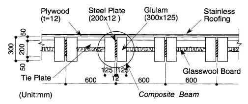
Fig.3 Section of Hanging Roof
