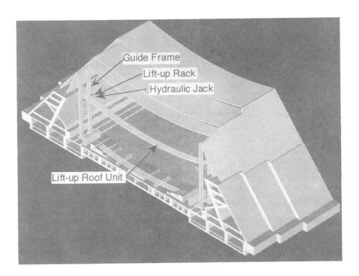
Fig. 4 Lift-Up Construction Method
