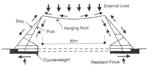
Fig.2 Basic Load Bearing Mechanism
