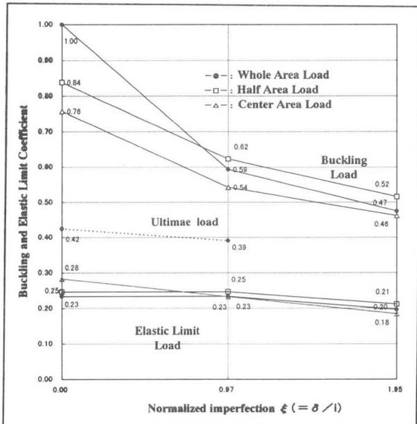
Fig. 2-1 Normalized imperfection amplitude and buckling coefficient
