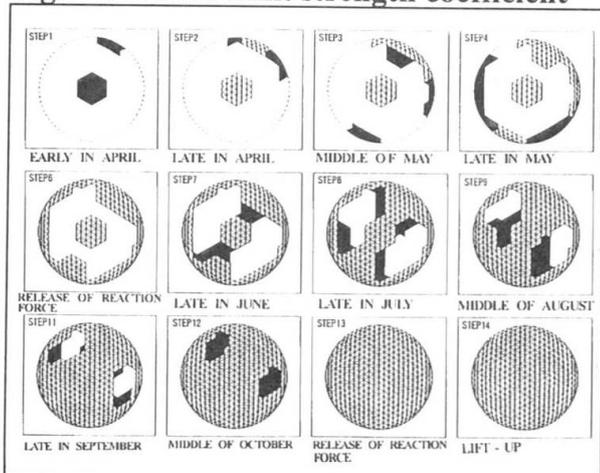
Fig. 3-1 Analytical models corresponding to construction steps
