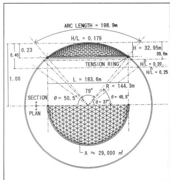
Fig 1-3 The roof Structure section
