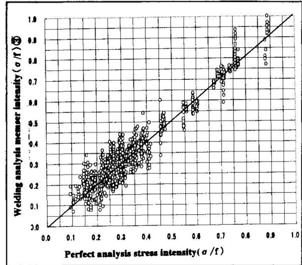
Fig. 3-4 Member stress intensity correlation (Welding analysis)
