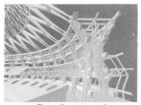
Fig.5 Grandstand Structure Supporting Dome
