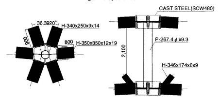
Fig.9 Cast Steel Node
