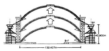
Fig.11 Lift-up Method Construction
