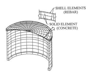
Fig. 4 Non-linear analysis model of underground tank
