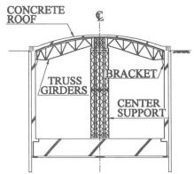
Fig. 9 Section of steel truss structure
