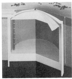
Fig. 1 General view of 200,000 kl LNG underground tank
