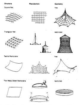
Fig. 12 Manufacturing double-curved light weight surfaces acting in tension.
