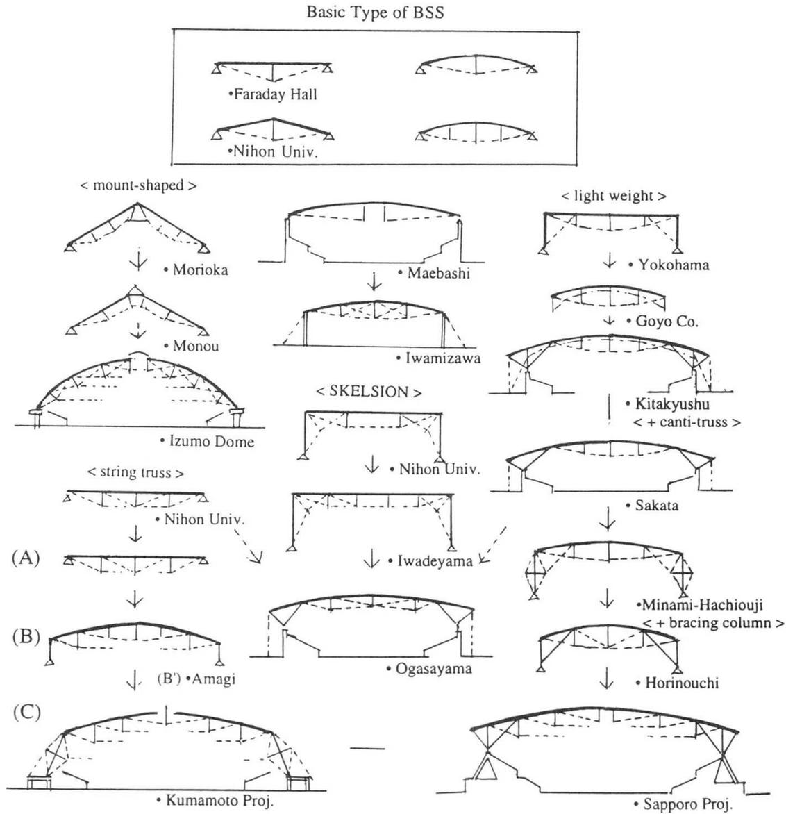
Fig.10 Various application from basic type of BSS
