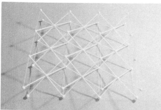
Fig.24 Model of Tensegric Truss unit
