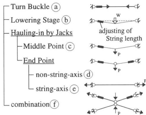
Fig.8 Method for introduction tensile force to string
