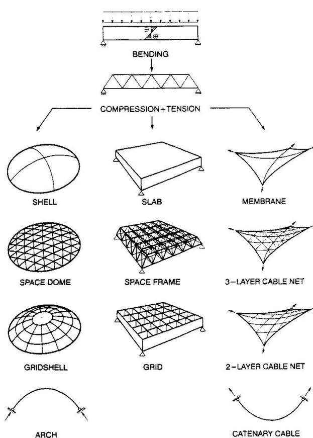
*Fig. 2 The development of double-curved surface structures.*
