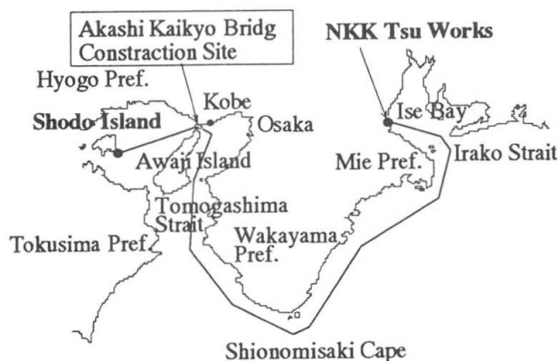
Fig.9 Towing route of 2P caisson
