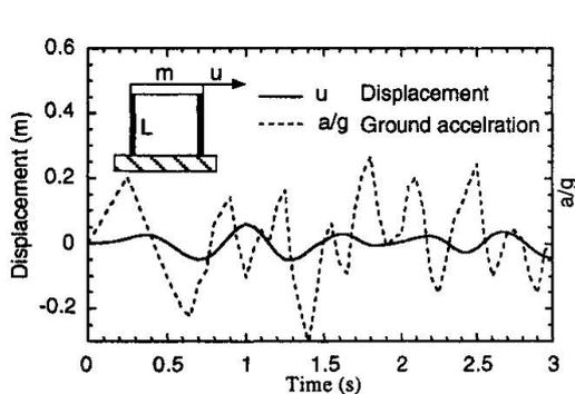
Fig. 3 Response of a simple elastic frame work subjected to ground acceleration.
