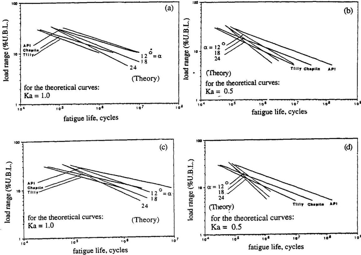
Fig. 4. Comparison of alternative design S-N curves for different values of  $K_a$ : (a) and (b)  $K_a = 1.0$  and  $0.5$ , respectively, for the fatigue life to first outer layer wire fracture; (c) and (d)  $K_a = 1.0$  and  $0.5$ , respectively, for the fatigue life to first wire fracture in the innermost layer.
