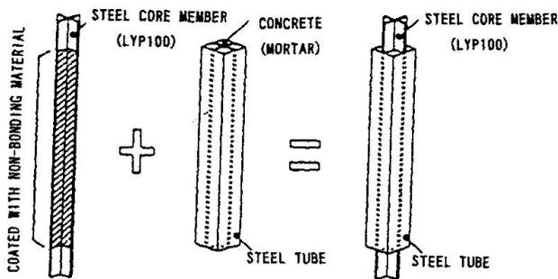
Fig 4 Unbonded Brace
