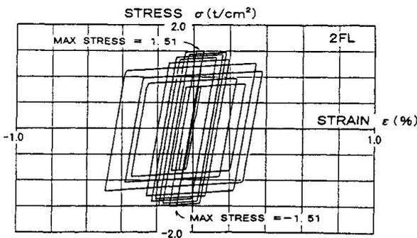
Fig 9 Stress-Strain Curve of Steel Core Member (50 kine)
