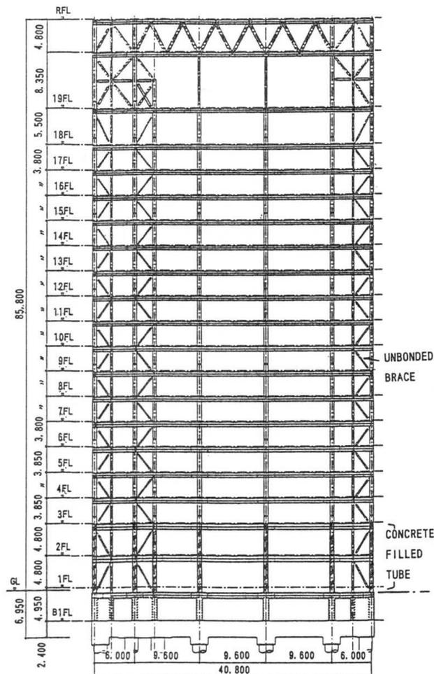
Fig 3 Framing Elevation ( N-S dir. )
