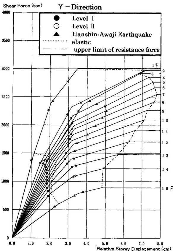
figure 4 Skeleton curve and Result of response analysis
