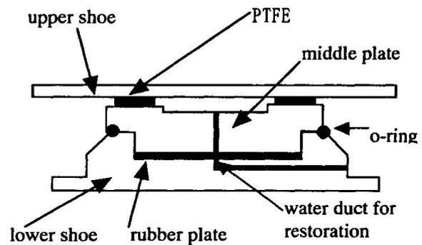
Fig. 2 Friction Bearing
