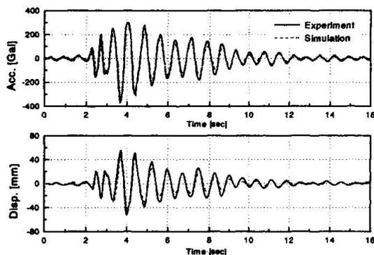
Fig. 13 Response of girder supported on rubber springs
