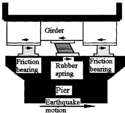
Fig. 1 Configuration of isolation system with friction damping
