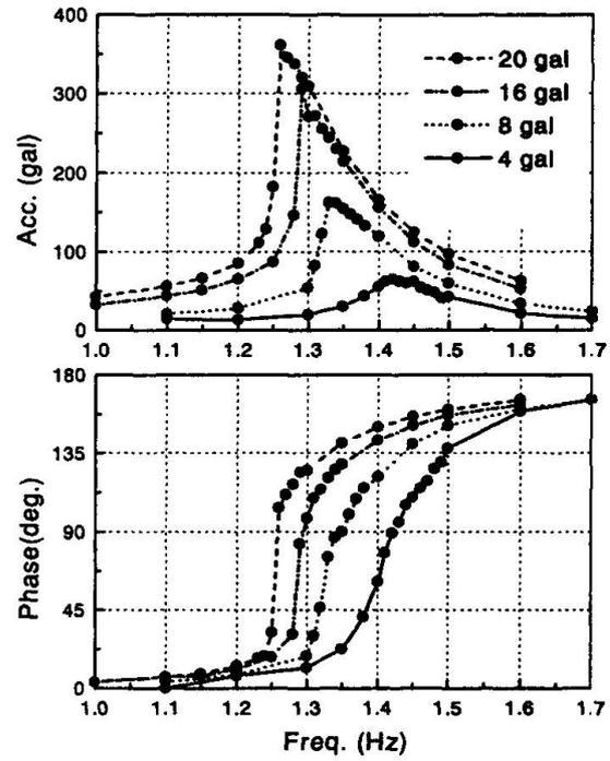
Fig.11 Frequency response of girder on rubber spring
