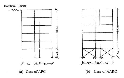
Figure 1, sketch for computational model of superstructure (unit: m)
