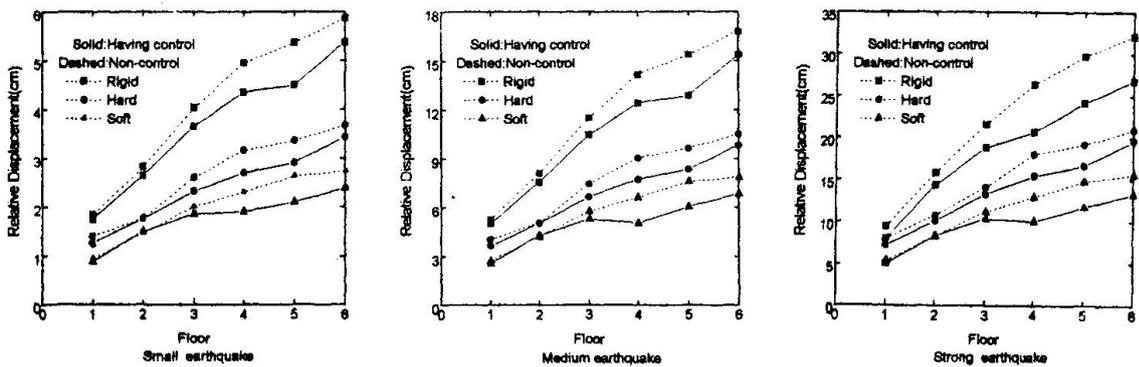
Fig.4 Comparison of relative displacement between non-control and APC for K=1000 kN/m
