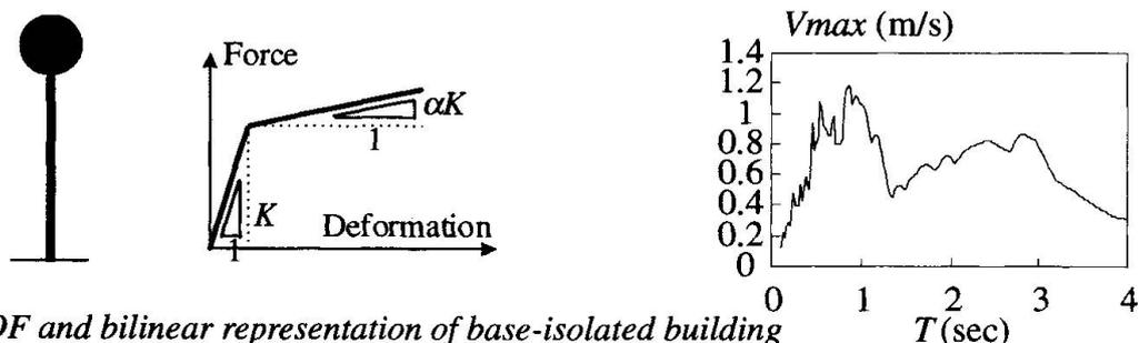
Fig.1 SDOF and bilinear representation of base-isolated building
