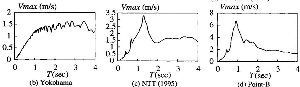
Fig.2 Elastic pseudo velocity spectra of ground motions analyzed
