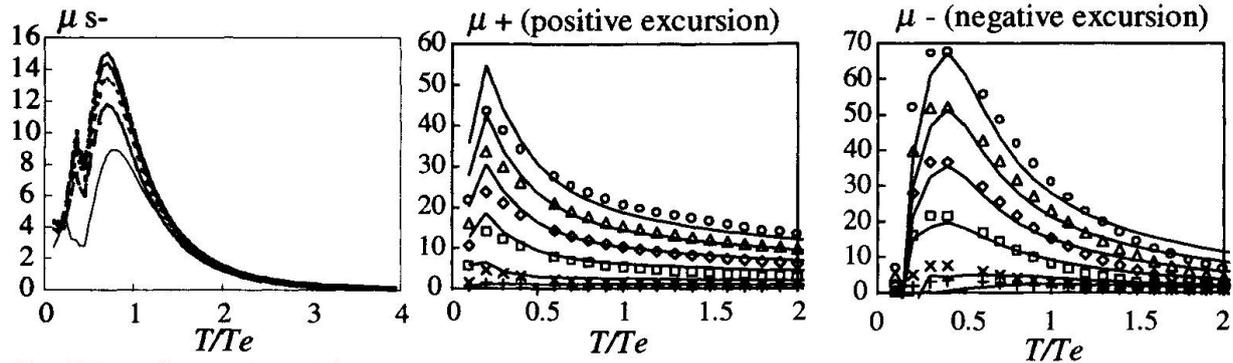
Fig.7 Ductility ratios with respect to static deformation
