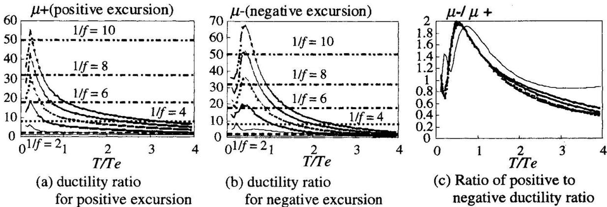
Fig. 6 Response characteristics of bilinear SDOF systems subjected to one-cycle sinusoidal ground motion
