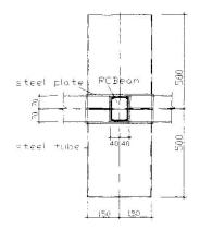
Fig.2: Beam-Column Joint Model
