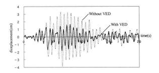
Figure 2. Time-history Diagram of Earthquake Response Analysis
