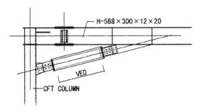
Figure 1. Detail Drawing of VED
