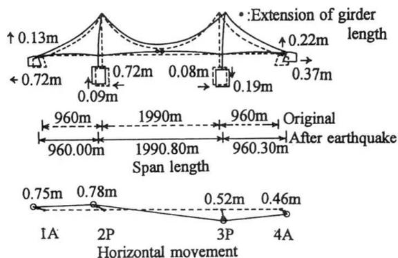
Fig. 7 Displacement of the Bridge after the earthquake
