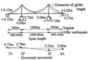
Fig. 7 Displacement of the Bridge after the earthquake
