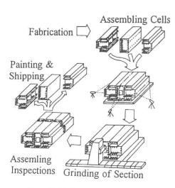
Fig. 2 Fabrication of tower shafts
