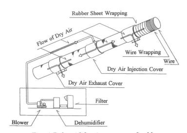
Fig. 4 Dehumidification system of cable
