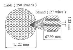
Fig. 3 Cross section of cable
