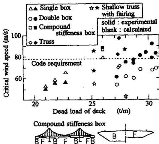
Fig. 5 Girder types and their flutter speed
