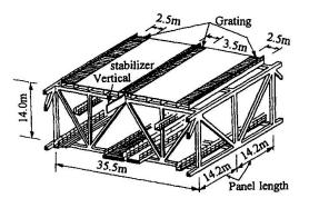
Fig. 6 Stiffening girder of the bridge
