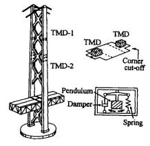
Fig. 1 Installation of Tuned Mass Damper
