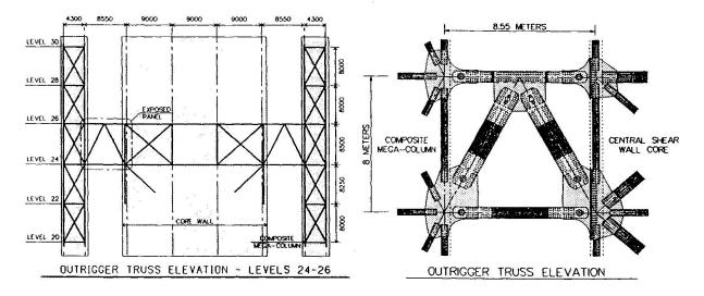
Figure 3 - Elevation and Detail of Outrigger Truss System
