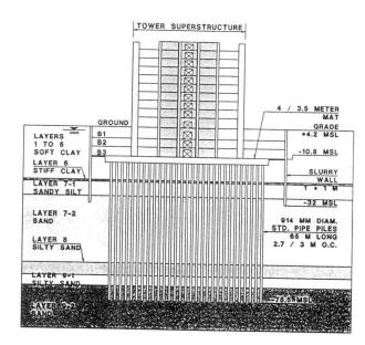
Figure 2 - Tower Foundation Systems
