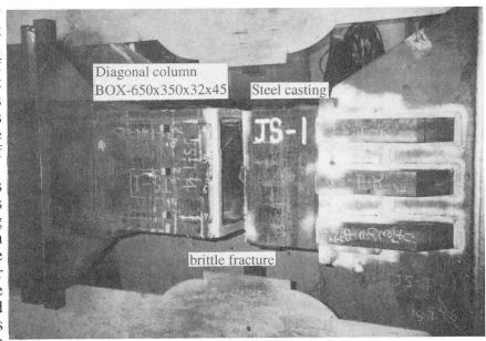
Fig. 10 Full-size test result of diagonal column joint
