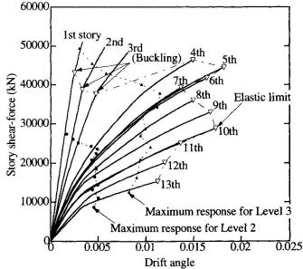
considerably short compared with general Fig. 4 Load-deformation curve and seismic response
