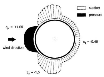
Fig. 8 Typical pressure distribution around the circumference of a cylindrical tube
