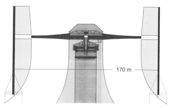
Fig. 6 200 MW vertical axis in the shaft of the solar chimney.
