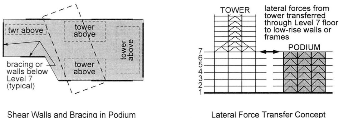
Fig. 11. Design concept with no expansion joints
