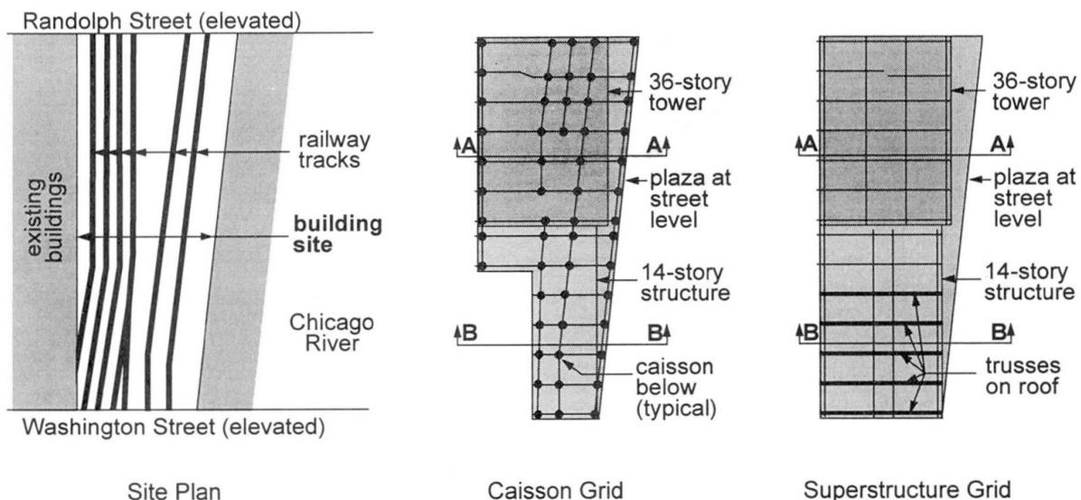
Fig. 4. Schematic layout of Morton International Building
