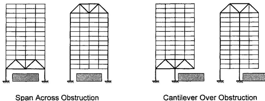
*Fig. 1. Structural transfer concepts for vertical load*
