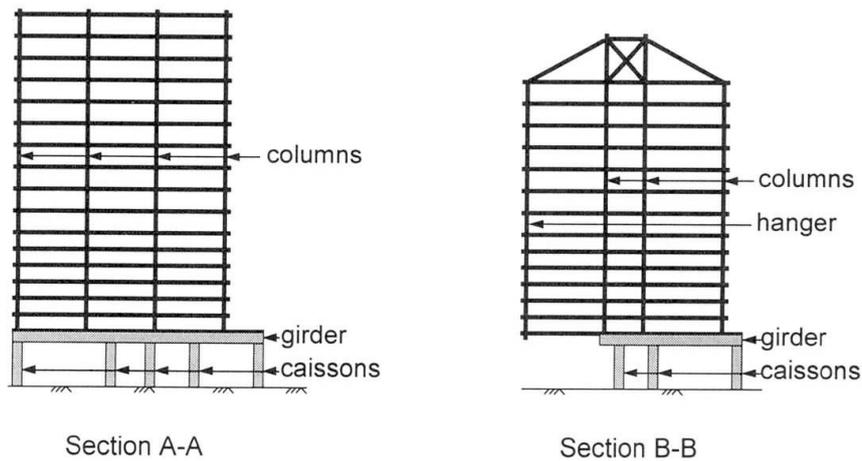
Fig. 5. Schematic sections through Morton International Building (see Fig. 4 for location of sections)
