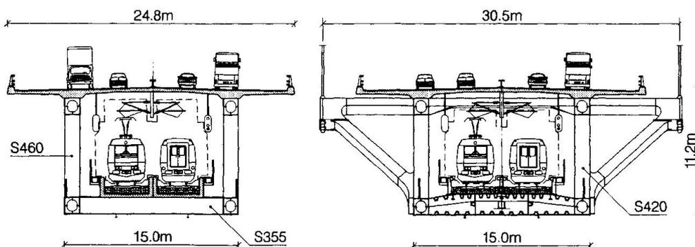
Fig. 4: Cross section of approach and high bridge, respectively
