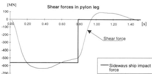
Fig. 1 : Dynamic shear force at level -17 m.
