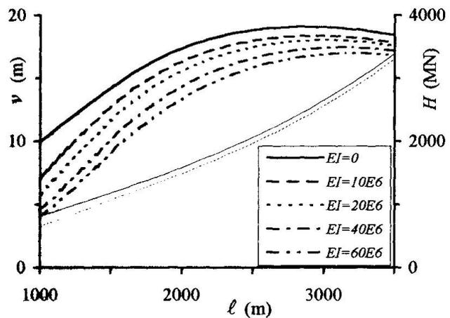
Fig. 2 Maximum displacement and horizontal tension versus  $\ell$
