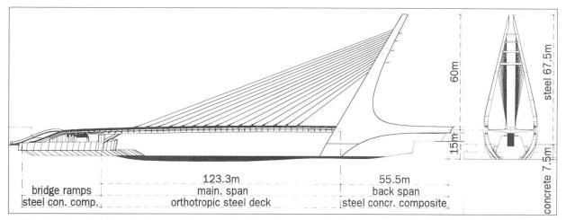
Fig. 1 Longitudinal view and cross-view-section
