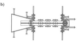
Fig. 1: Modern modular expansion joint
