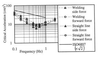
Fig. 5: Limits of straight line drawing or welding tasks
