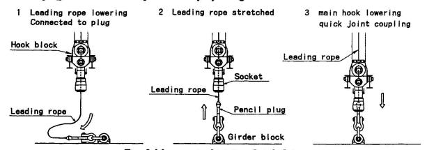
Fig. 2 Movement of joining Quick Joint
