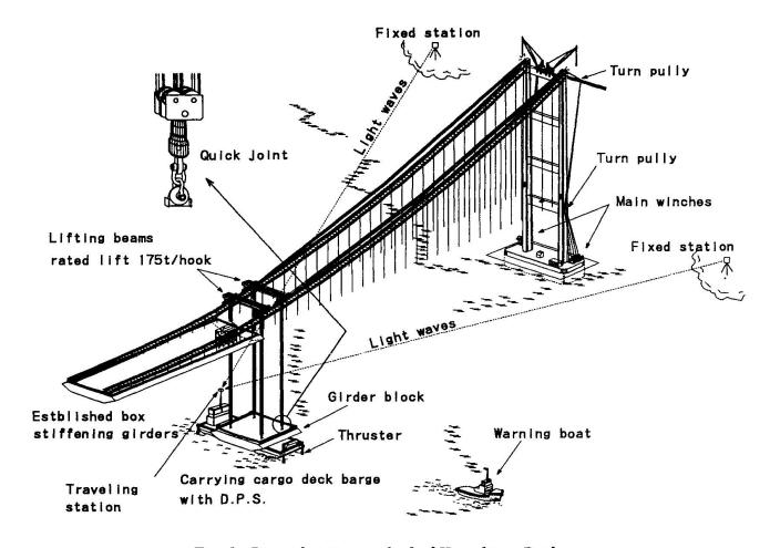
Fig. 1 Direct hoisting method of Kurushima Bridges
