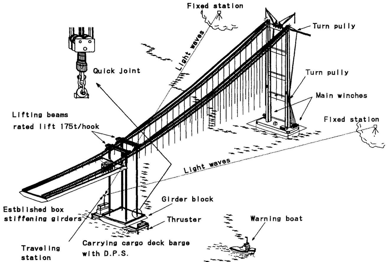
Fig. 1 Direct hoisting method of Kurushima Bridges
