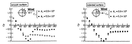
Fig.-4 Pressure Distribution of Cables
