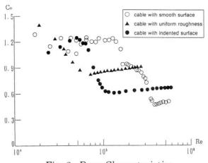
Fig.-3 Drag Characteristics
