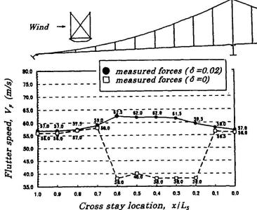
Effects of cross stays on flutter speed Fig.3(Case-S) Œ measured forces (\$\delta\$=0.02) 80.0 measured forces ( $\delta = 0$ ) Theodorsen's forces ( $\delta = 0$ ) (s/m)Flutter speed, V, 85.0 40.0 35.0 0 25 0.40 0 20
