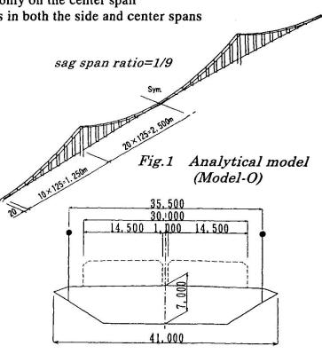
Fig.2 Section of girder
