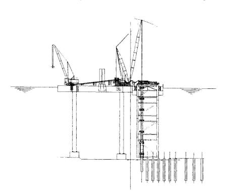
Inclusions driving with the tension leg platform
