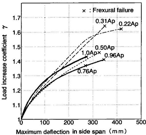
Fig.5 Relationships between load increase coefficient and girder deflection
