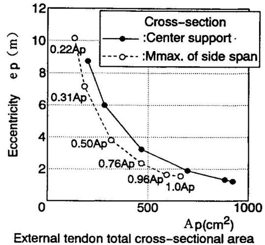
Fig.2 Relationships between total external tendon cross-sectional area and eccentricity in major cross-sections for each model
