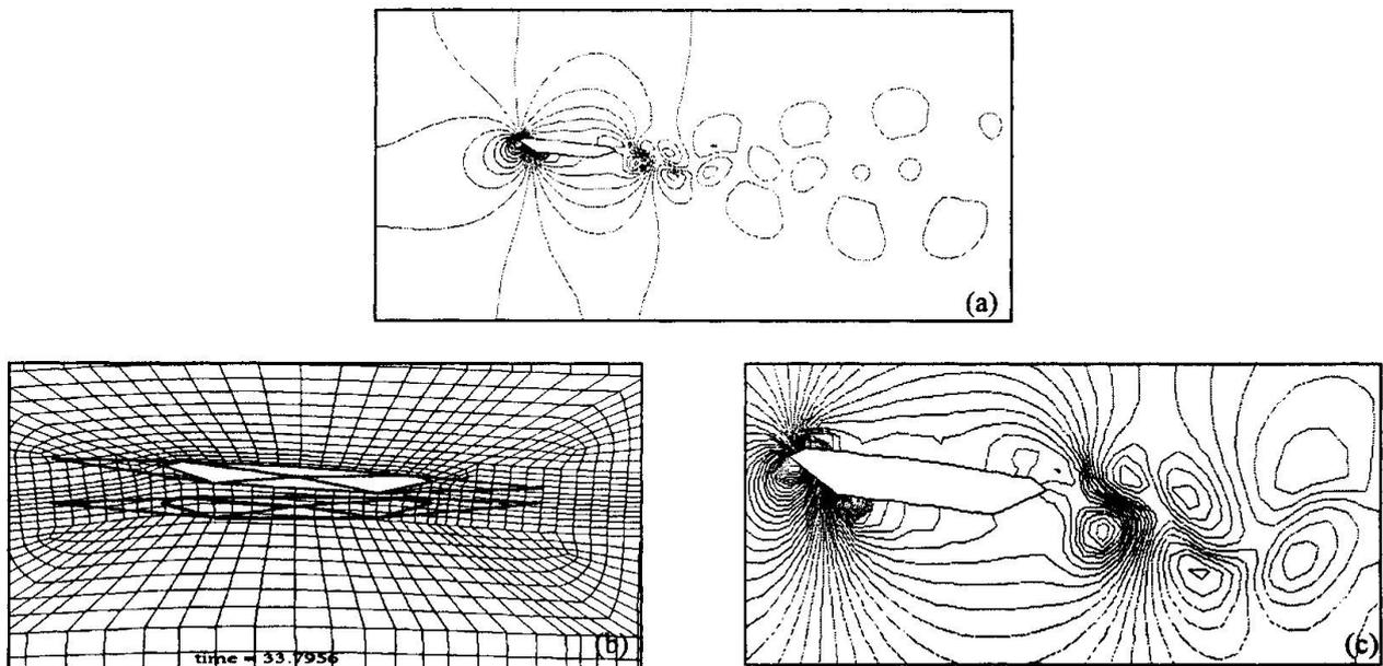
Fig. 7. Coupled flutter at 60 m/s. (a) Pressure contours in whole domain. (b) Mesh deformation (c) Pressure contours near deck. (displacements magnified 5 times).
