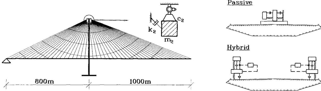
Fig. 5 : Cable-stayed bridge under construction (main span 2000m)
