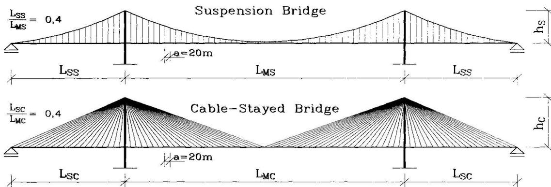
Fig. 2 : Suspension and cable-stayed bridge systems with fan-shaped cables
