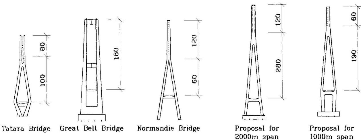
Fig. 4 Types of pylons
