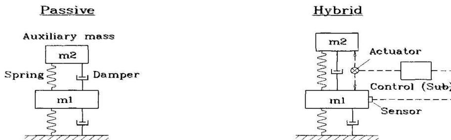
Fig. 6 : Tuned mass dampers
