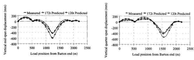
Figure 3 - Single Heavy Lorry Crossing - Comparison of Measured and Predicted Vertical Displacements at a) Midspan b) Quarter Point of Centre Span
