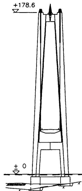
Fig. 6. Pylon elevation.
