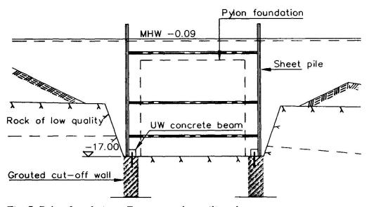
Fig. 7. Pylon foundations. Temporary sheet piling shown.
