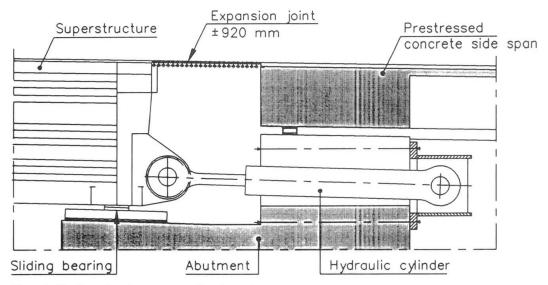
Fig. 4. Hydraulic dampers at bridge abutments reducing longitudinal movements to  $\pm 0.85$  m.
