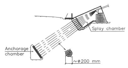
Fig. 5. Main cable anchorage.
