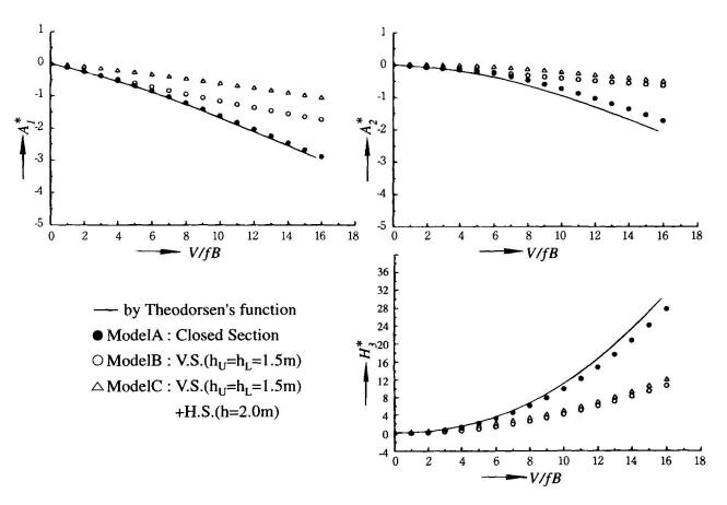
Fig. 5 Examples of Flutter Derivatives (Model A, B, C)
