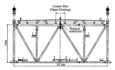
Fig. 1 The Vertical Stabilizer of the Akashi-Kaikyo Bridge in the center span
