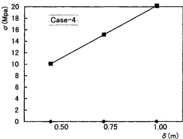
Fig 11. Extra stress in the suspended girder
