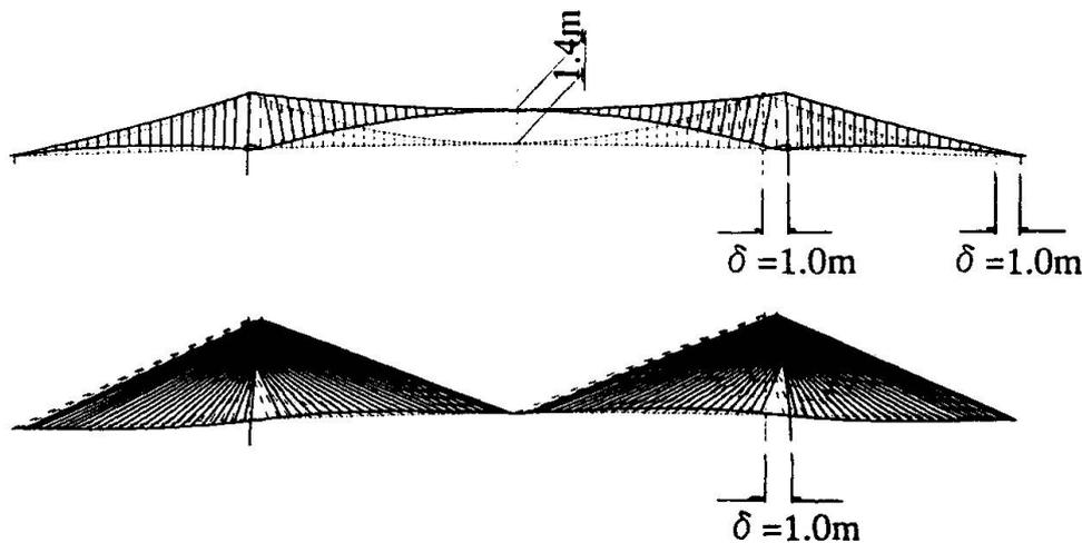
Fig 3. Bridge deformation
