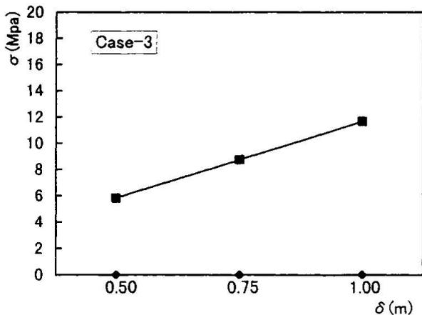
Fig 9. Extra stress in the suspended girder
