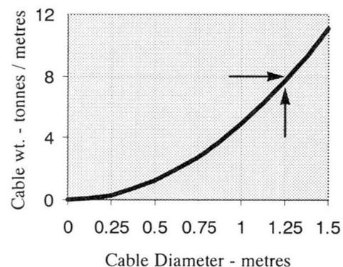
*Fig 1 - Relationship of Cable Weight & Diameter*
