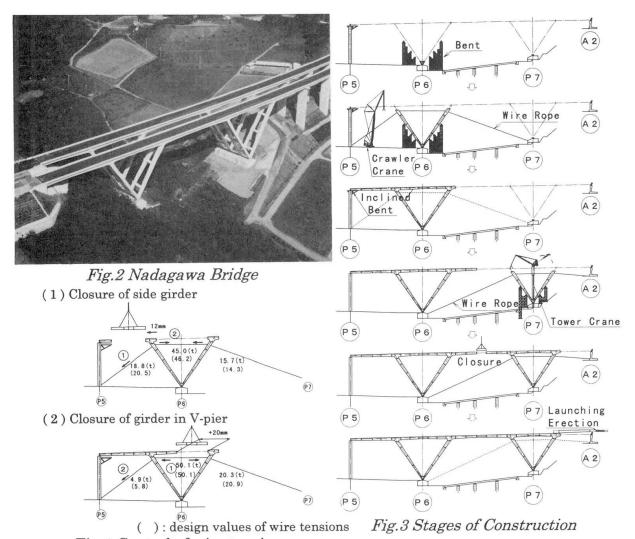
Fig.4 Control of wire tensions
