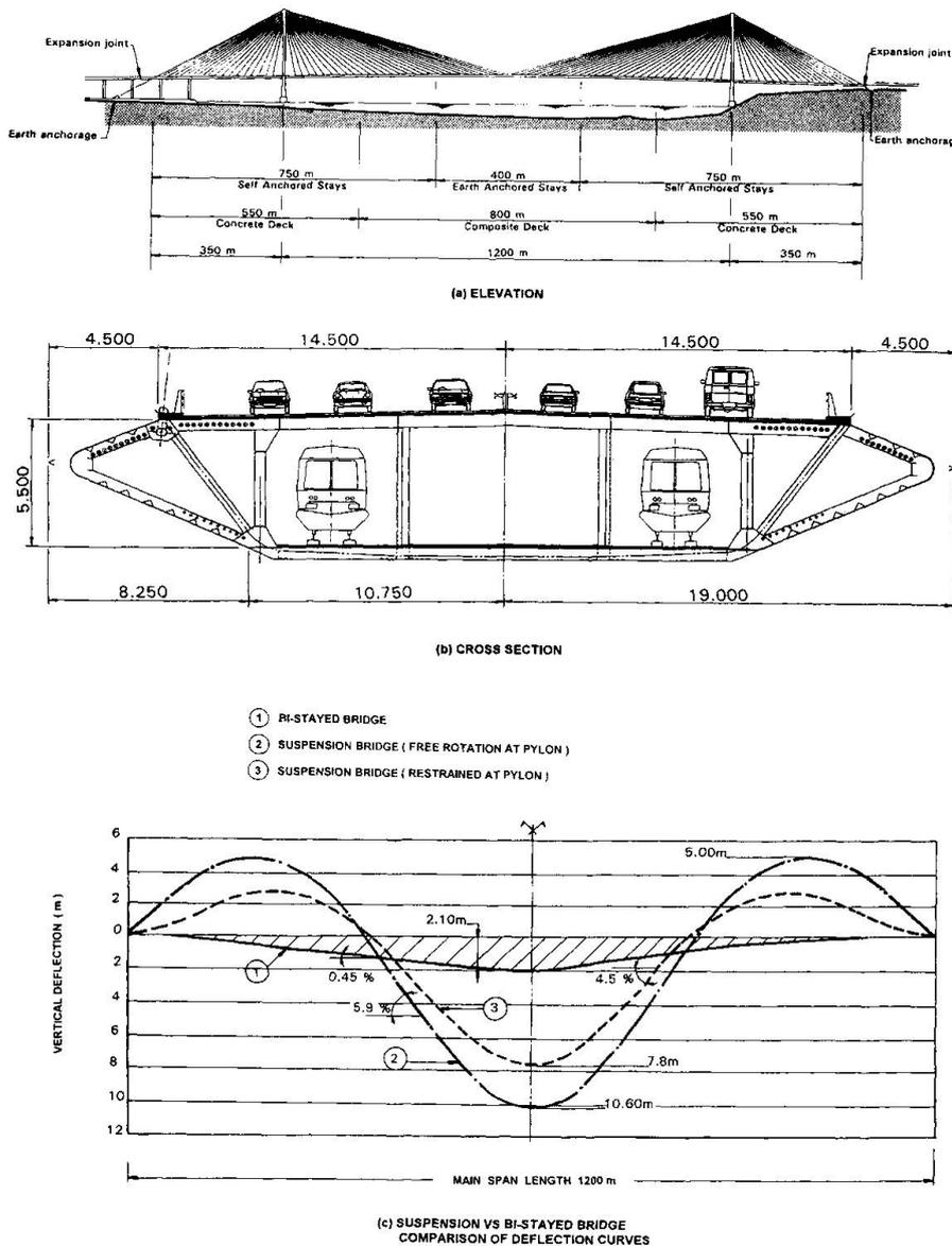
Fig. 6 Example of 1,200 m. Bi-stayed Bridge
