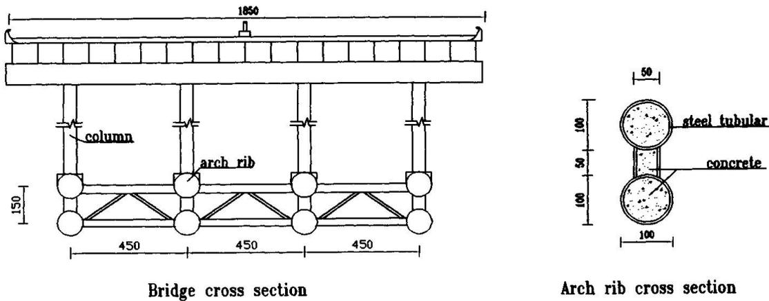
Fig.3 Arch bridge structure cross section
