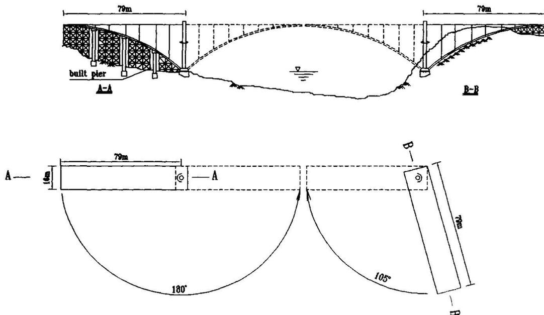
Fig.4 To rotate the arch rib
