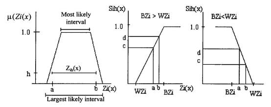
Fig. 2 Fuzzy calculation of basic criteria Fig. 3 Transfering value  $Z_{ih}(x)$  into  $S_{ih}(x)$  Because of the units of the basic criteria are different, since for some the best value is the highest while for other is the opposite (the best price is the lowest and the best constructive yield the highest), the value of each basic criterion  $[Z_{i,h}(x)]$  in Fig. 2 is transformed into a index  $S_{i,h}(x)$  in the following way [6]:
