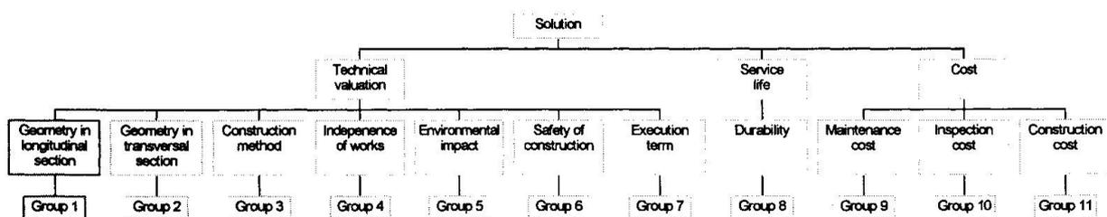
Fig. 1 Diagram of deck bridge basic criteria (see Table 2)
